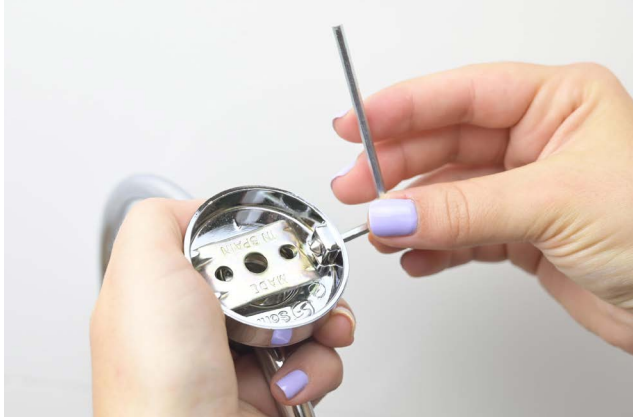
1. Remove the back plate.
