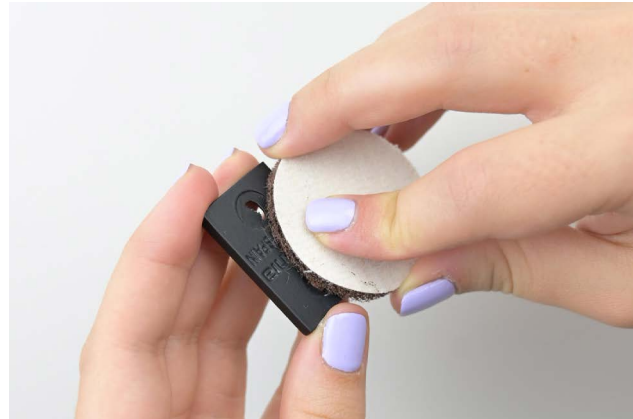
2. Sand the back plate surface.
